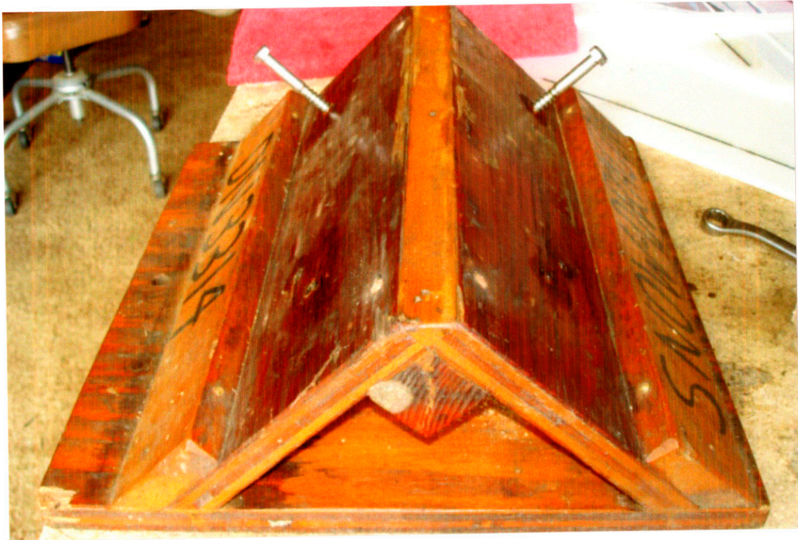
JIG FOR SHARPENING RUNNERS, ADAPTED FROM DN
