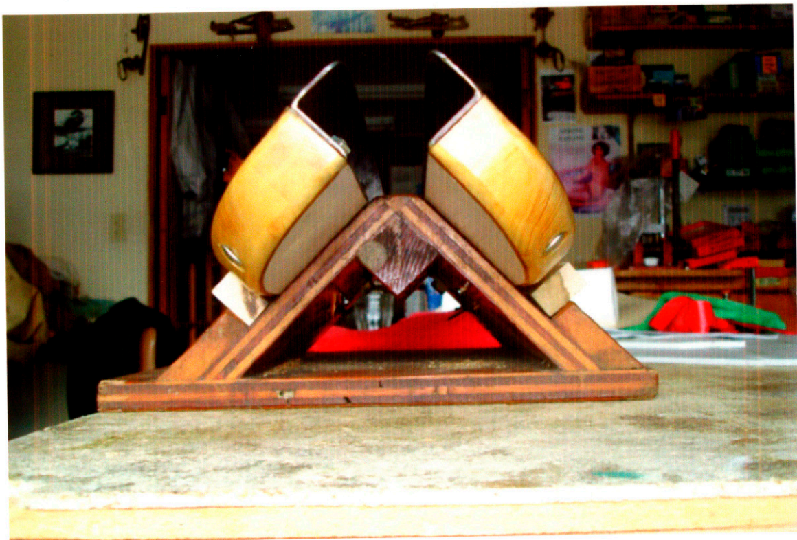
RUNNERS ON JIG TO SHARPEN OUTSIDE EDGES
